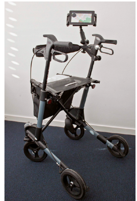
The Navigation Aid user interface runs on an Android Nexus-7 tablet, and is mounted on a commercially available TOPRO TROYA walker.
